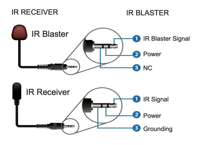
Note: When the angle between the IR receiver and the remote control is  $\pm 45^{\circ}$ , the transmission distance is 0-5 meters; when the angle between the IR receiver and the remote control is  $\pm 90^{\circ}$ , the transmission distance is 0-8 meters. the angle between the IR receiver and the remote
